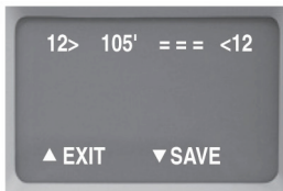
Figure 6-46. A wire map for a coax cable.
